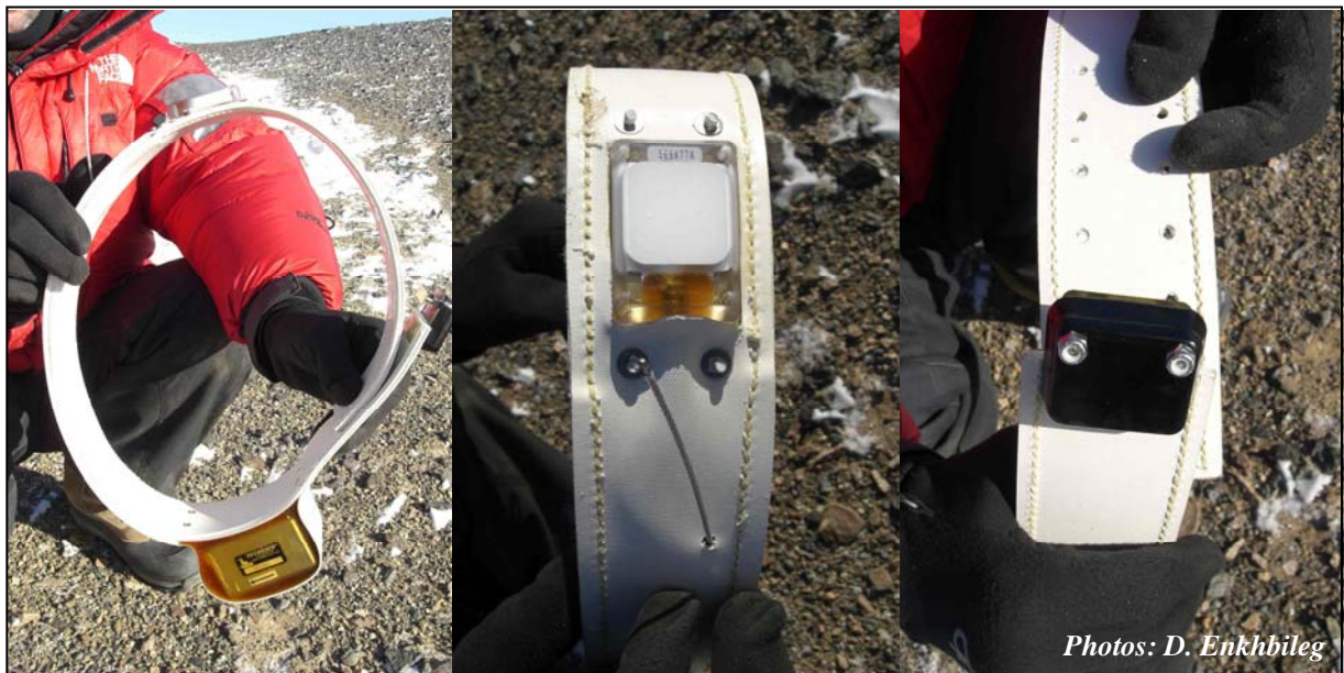
Fig. 13: a. Wild camel collar TGW-3580 from Telonics, b. GPS Antenna (square) and ARGOS antenna (rod), c. CR-2a drop-off.
